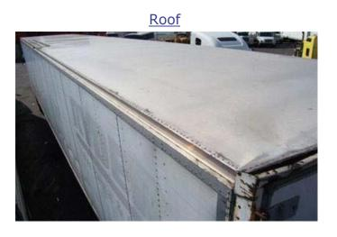
New Rivets / Repairs
