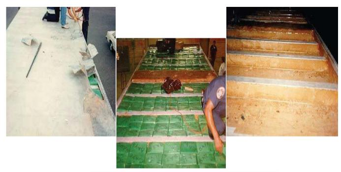
False Trailer Roof / Orginal Rivets Removed
